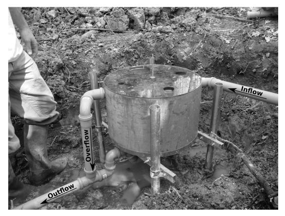
Figure 2.2: Fully assembled and installed WME with foundation poles. The holes in the lid of the WME are for the placement of the measurement sensors.
