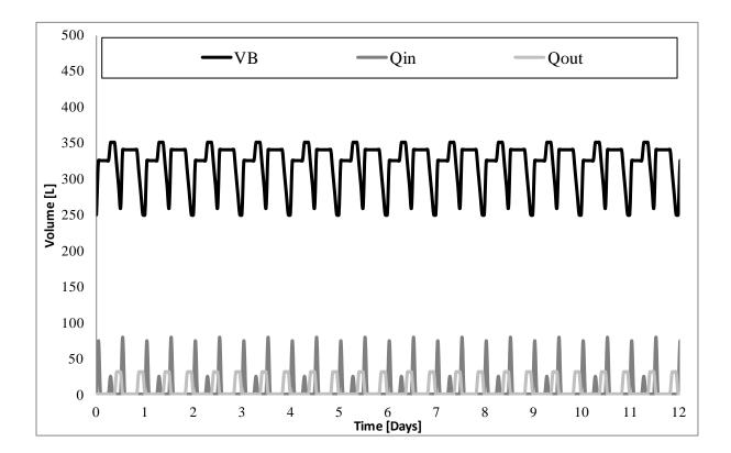
Figure 5 - 1: Modelled hydraulic characteristics of bioreactor volume (V<sub>B</sub>), inflow (Q<sub>in</sub>) and effluent (Q<sub>out</sub>)
