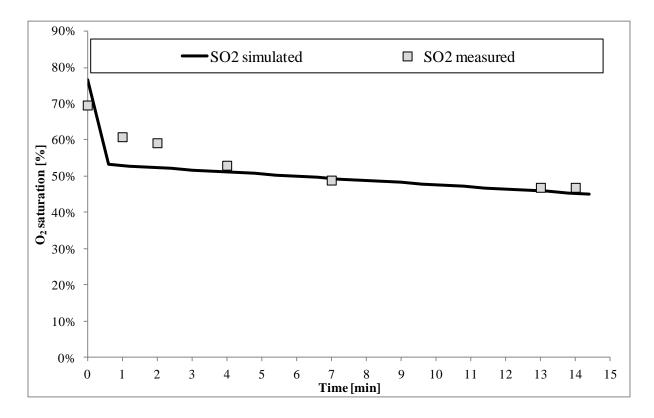
Figure 5 - 3: Oxygen saturation decay in the bioreactor with switched-off aeration blower shortly after feeding fresh grey water. The straight line shows a comparison between modelled and measured  $O_2$ -saturation.
