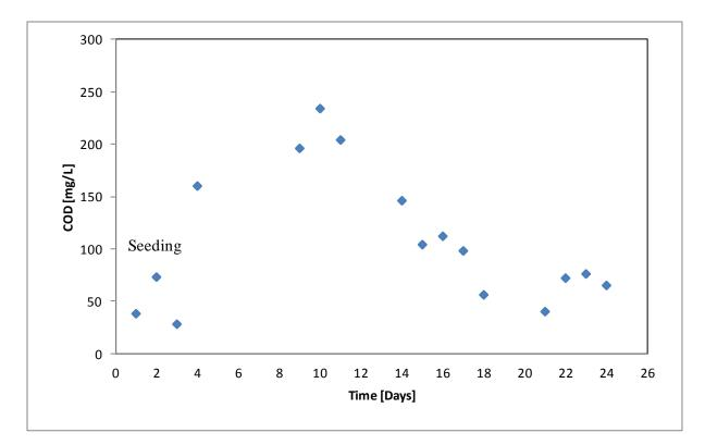
Figure 3 - 2: COD development in treated water after start up with seed microorganism
