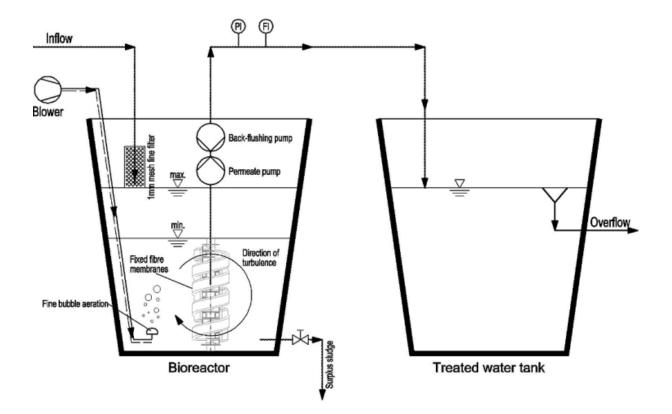
Figure 4 - 1: Schematic diagram of the fixed-fibre biofilm membrane pilot plant
