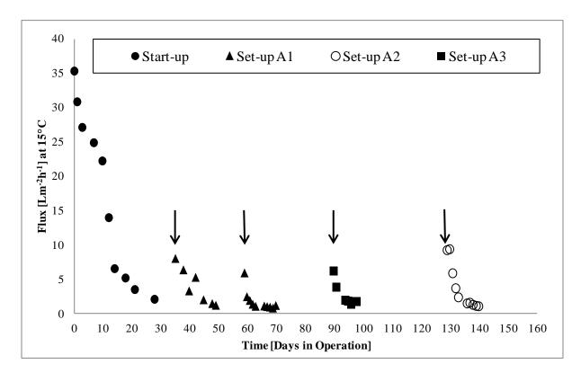
Figure 4 - 4: Flux stabilization after start-up (0.38 Lm-2min-1) and at different aeration rates (A1 0.19 Lm-2min-1, A2 0.38 Lm-2min-1, A3 0.67 Lm-2min-1), temperature corrected to 15°C, arrows indicate out-of-tank washes of membrane module.
