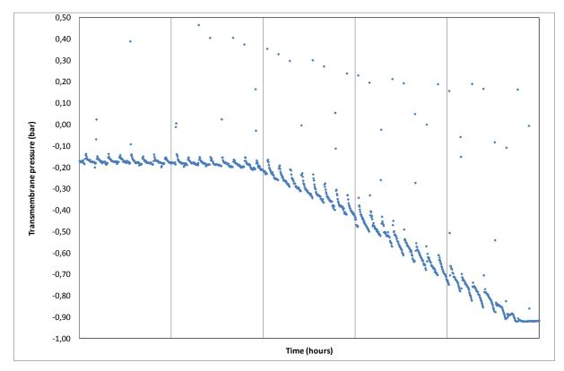
Figure 2 - 2: Transmembrane pressure (TMP) during constant flow operation without back-flushing
