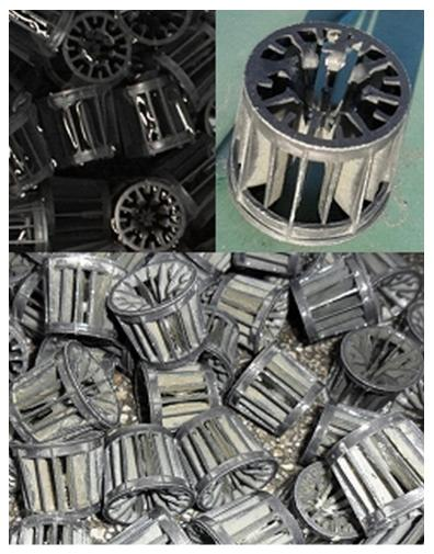
Figure 3 - 7: Comparison of the biofilm thickness and structure between after start-up (top left), week 5 (top right) and week 20 in operation.
