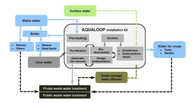
Figure 2: Flow scheme of Aqualoop treatment system from company Intewa
