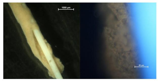
Figure 4 - 5: a) Stereo-microscopy of membrane fibre with biofilm-cover; scale bar represents 1000 μM;
