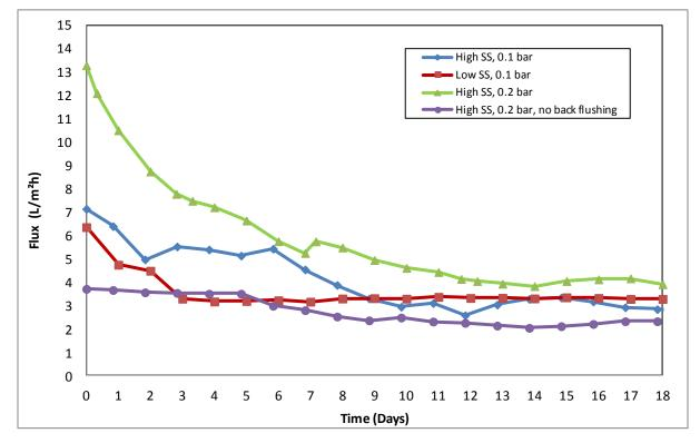
Figure 2 - 3: Flux development during three weeks operation with different TMP and suspended solid (SS) concentration
