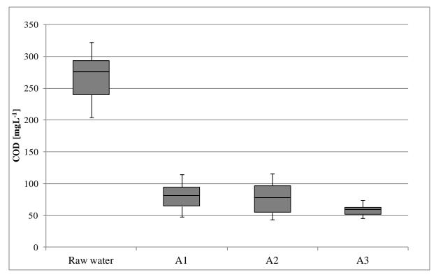
Figure 4 - 3: COD removal efficiency depending on aeration rates (A1 0.19 Lm-2min-1, A2 0.38 Lm-2min-1, A3 0.67 Lm-2min-1). Bar chart analyses of each set-up including median, 25% and 75% quantile and whisker.
