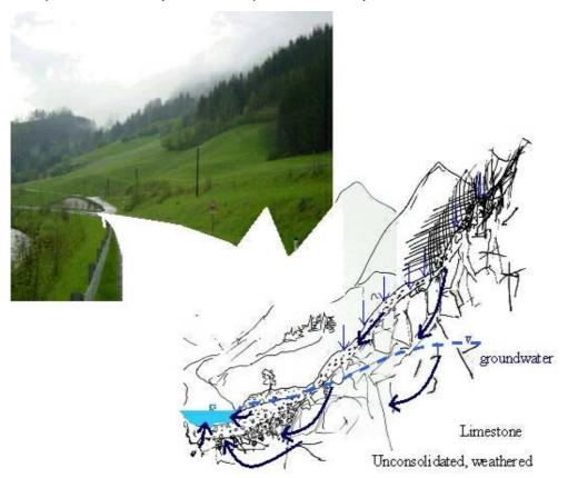
Fig. 2-2: graphical model 1of the upper Ybbs catchment, unconsolidated rock
