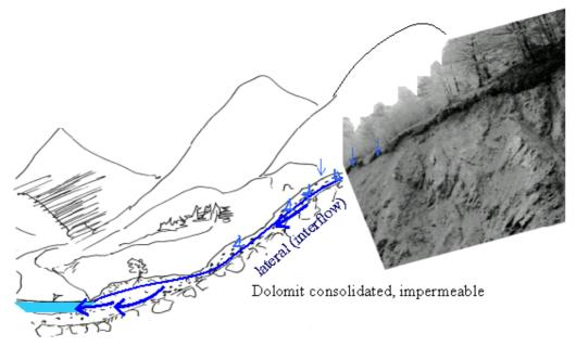
Fig. 2-4: graphical model 2 of the upper Ybbs catchment, consolidated rock
