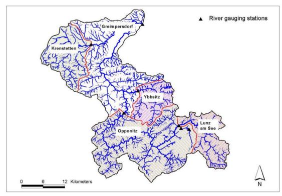
Fig. 2-15: Subcatchments and the location of the gauging stations in the Ybbs catchment
